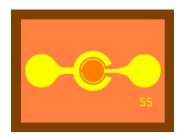
This high-performance product is a front side illuminated InGaAs PIN photodiode chip that features a large  $55\mu m$  detection window, and two large flexible wire-bonding pads. This product has low capacitance, high responsivity, low dark current and excellent reliability, designed for long wavelength optical receiver applications with date rate up to 10Gbps at wavelength from 1200nm to 1600nm with an either single mode or multi-mode fiber.
